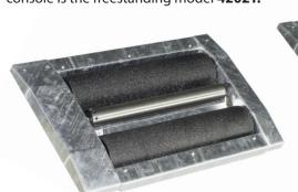
As standard, both rollers on the RT5204AB are **raised** and is equipped with a power box with a **double soft starter.** Soft starters gradually increase the power to the brake tester motors during start-up. This makes this unit suitable for testing in the applied brake testing mode. Also standard are the electronic motor brake, automatic slip detection, emergency stop and ON/OFF light indicator.
